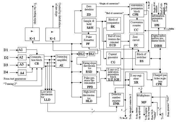
The whole information coming from the above described analyzers and intensimeters is memorized in the RAM device in a given sequence, depending on the character of the observed X-ray phenomena. By a command transmitted from the satellite's service system, the information is reformatted and translated to the onboard type recorder. After transmitting the whole information, the device automatically starts working in the mode transmitted by the ground-based station and written in the command memory.
